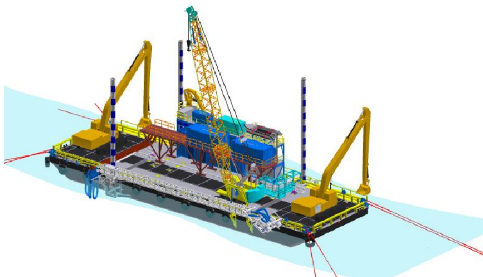
Figure 8.1.3 UB-01 with 90T crane and Trailing Arm (standby) support for shallow water pre-trenching using mooring winches (Illustration)
