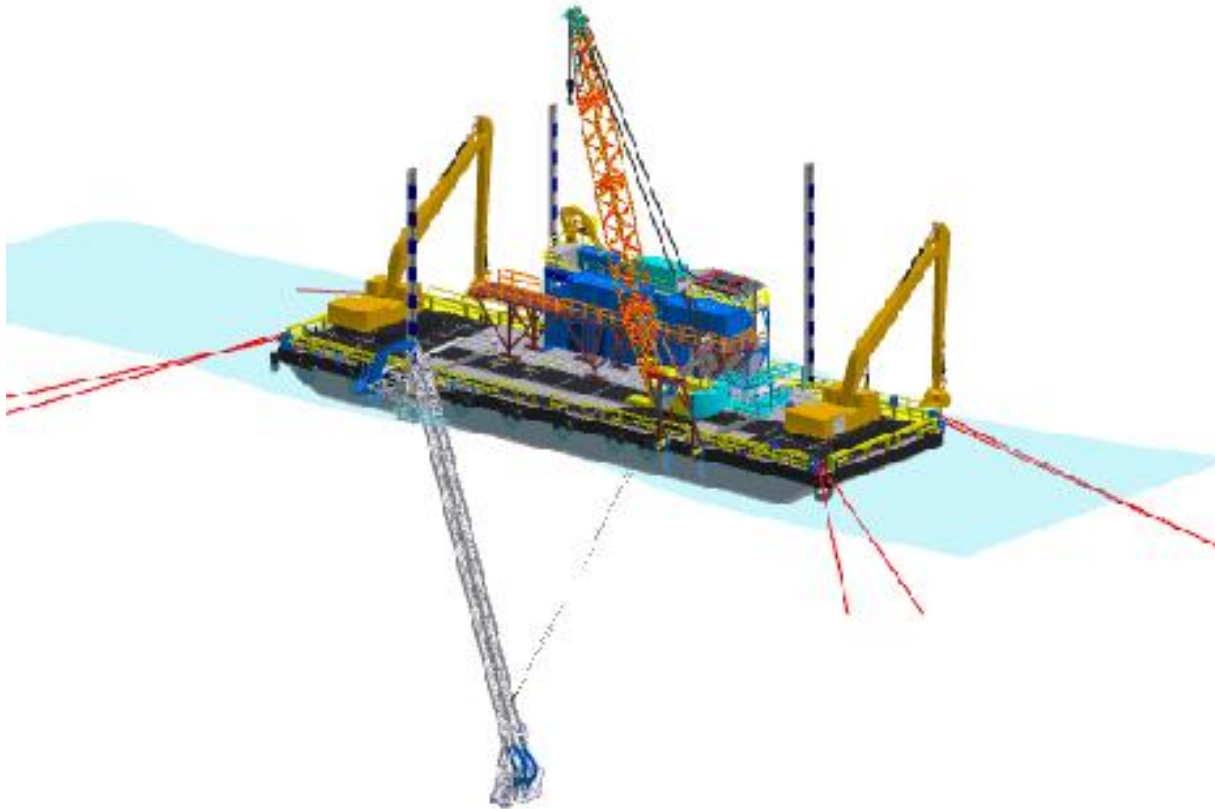
Figure 8.1.4 Configurations for UB01 Ms Pennie with Trailing Arm for Pre Trenching (Illustration)
