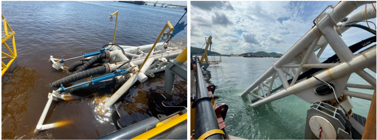
Figure 8.5.8 Trailing Arm Components (Arm and top support section)
