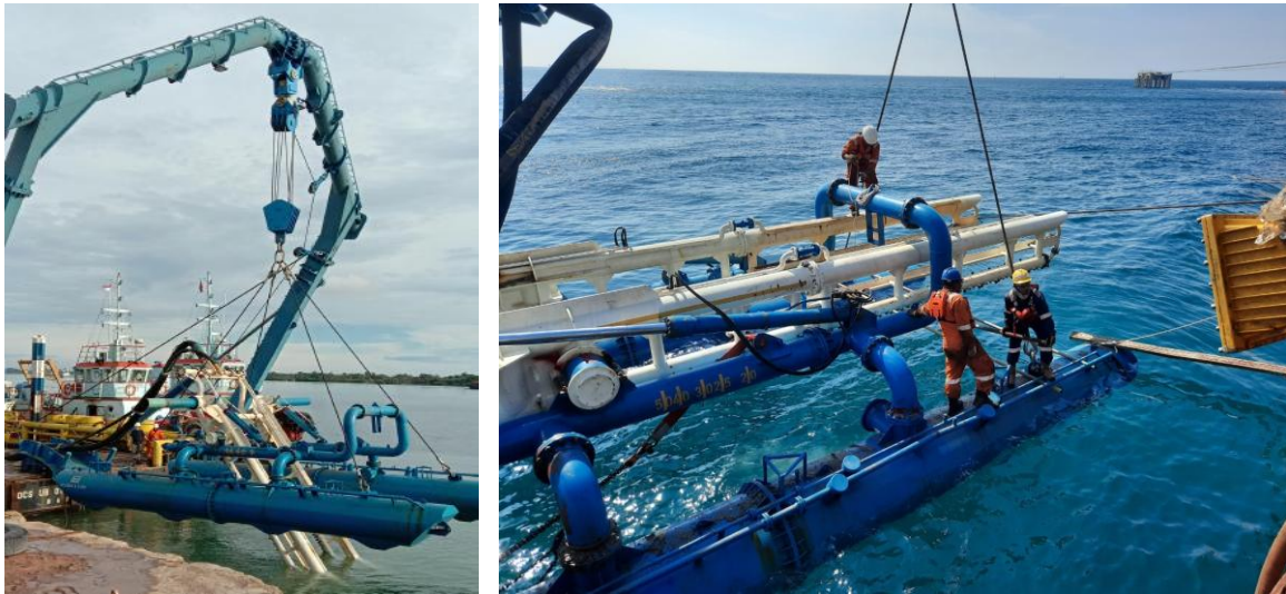
Figure 7.2 Articulated Jet Sled in operation mode
