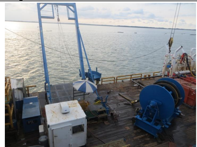
A-Frame boom out/set up over side of barge with spooler
