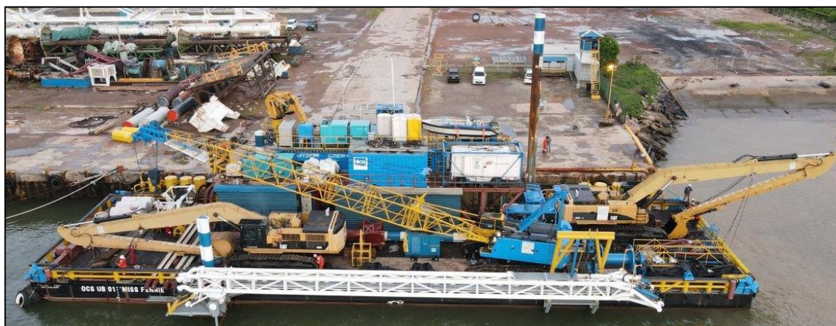
Figure 7.4 Trailing Arm pre-installed on UB01
