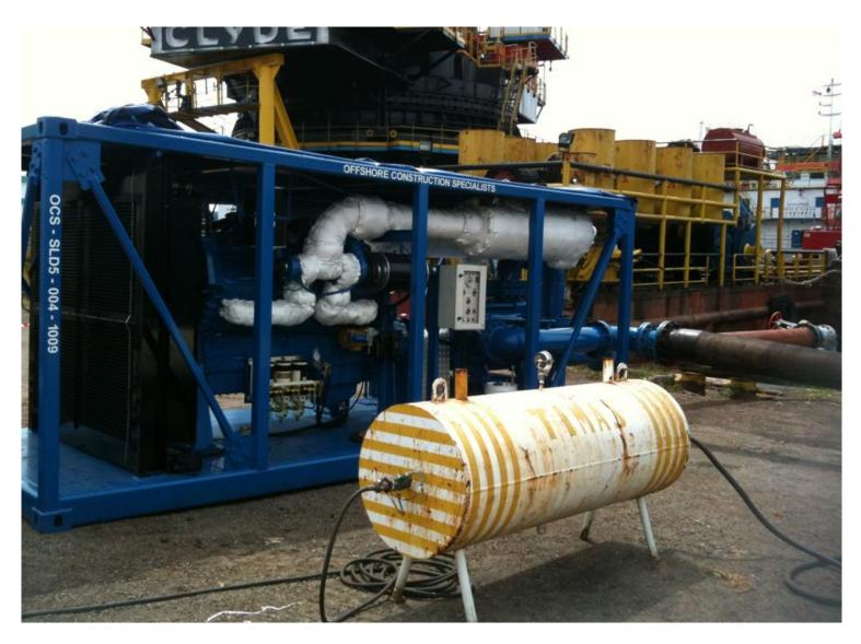
OCS owned 4 staged pump (12V149 engine driven) units are skid mounted pumping unit that can be used for high pressure water. Main type of operations performed using these units are pipeline precommissioning, Pipeline post burial (Trenching) and Pile remedial operations using Jet/Airlift techniques.
