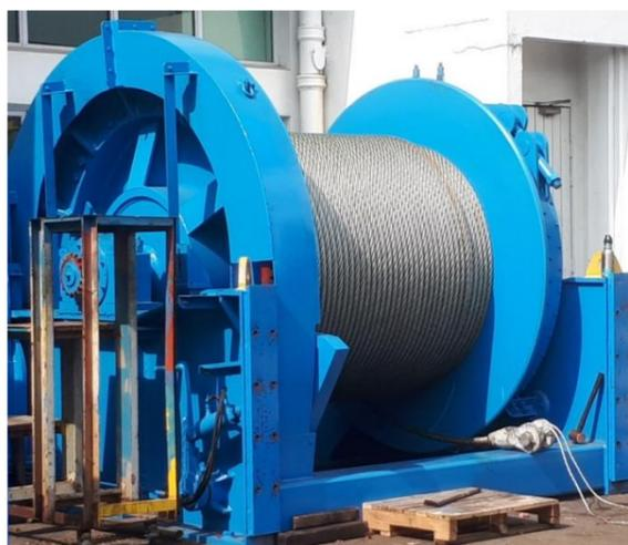
OCS's 60T Hydraulic Single Mooring Winch is used for pipe pulling operations. The winch comprise of a drum which is welded to a high tensile steel main shaft supported by a pair of bushing/bearing. A central pinion shaft is mounted on drive shaft and fitted with jaw clutches to allow drum to work. The drum is also fitted with a spring loaded and hydraulic release fail-safe band brake.
