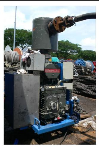
The Edwards vacuum pump employed in the OCS's pipeline pre commissioning operation spread is Edwards model E1M 275 vacuum Pump with Edwards EH1200 series mechanical booster pump.
