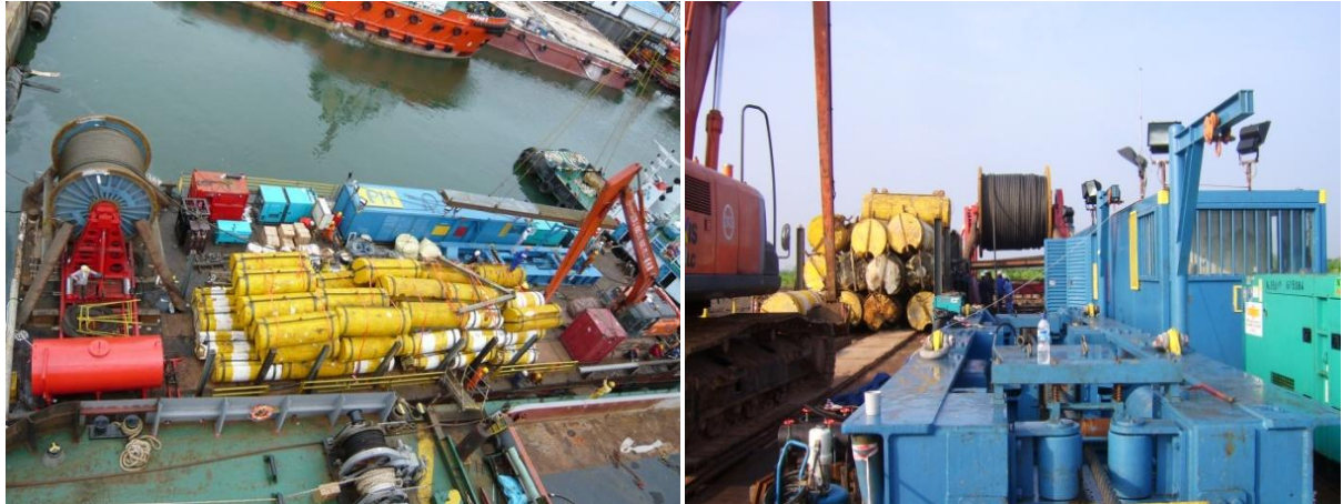
Figure 4.4.2 Lucker winch/Spooler can also be set up on the barge (pull barge option)
