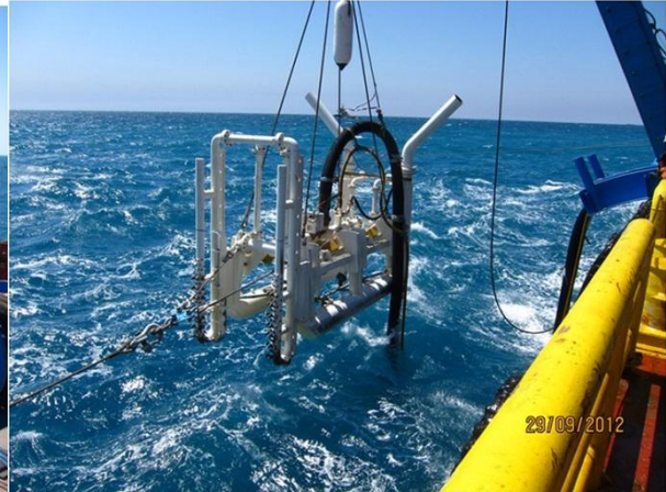
Jet Sled Being Lowered onto Pipeline
