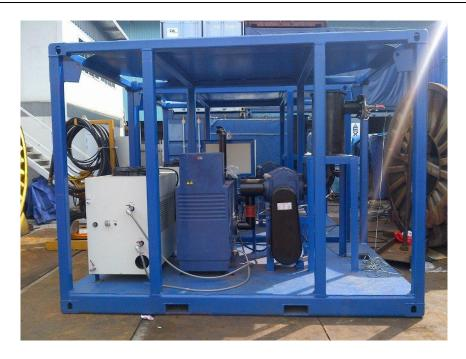
The Stokes vacuum pump employed in the OCS's pipeline pre commissioning operation spread is Stokes model 412-11 Microvac Pump with stokes 615M series blower.
