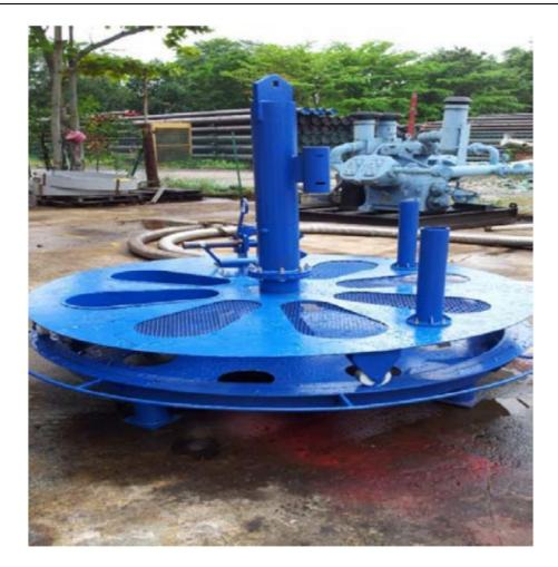
The ROV Installation turn-table is utilized to deliver Fabric formwork (Grout Bags) to seabed on freespan rectification projects where Remote Operated Vehicles (ROV) is the preferred system for installation.
