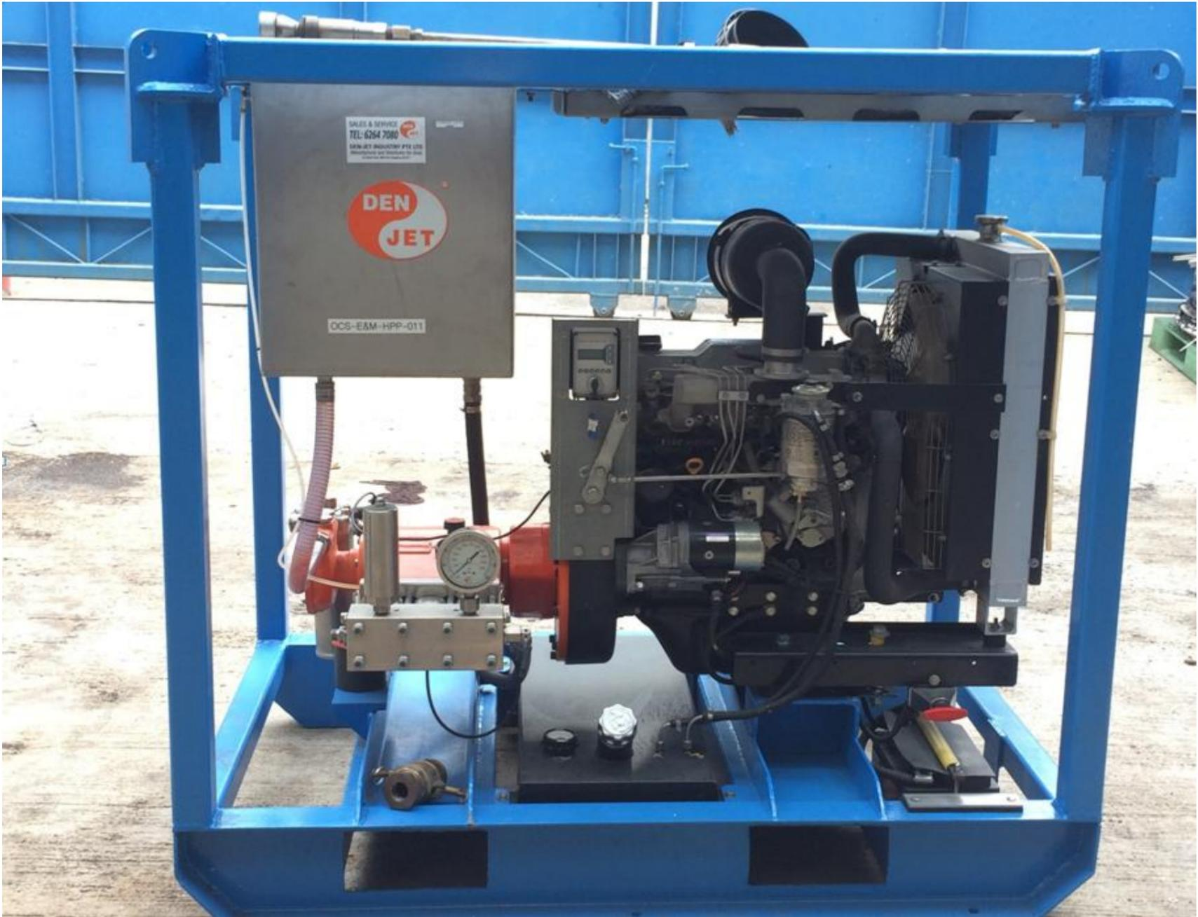
*OCS owned Denjet pump is skid mounted pumping unit, which is used for hydro static testing of subsea pipelines and also for the high pressure water blasting cleaning purposes. This pump is a normally used for hydrostatic testing of pipelines with high pressure requirements. OCS's owns two CD50 series Denjet pump skids. One pump skids is CD50-500 series with an operating pressure of 500bar (7250psi) and the other one is a CD50-1250 series with an operating pressure of 1250bar (18130psi).*
