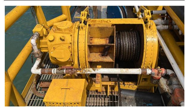
OCS's AIR driven 10 Ton maxpull winches are general multipurpose winches.
