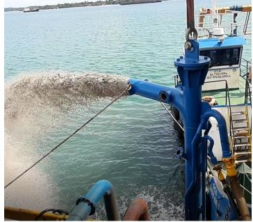
OCS designed and built jet / airlift combined with our unique high pressure / volume Pump skids and compressor are used for Pile plug removal. The pumps generate 2000 USGPM at 600psi. A two stage 1070 cfm x 350 psi compressor and all required hoses and fittings completes the spread.
