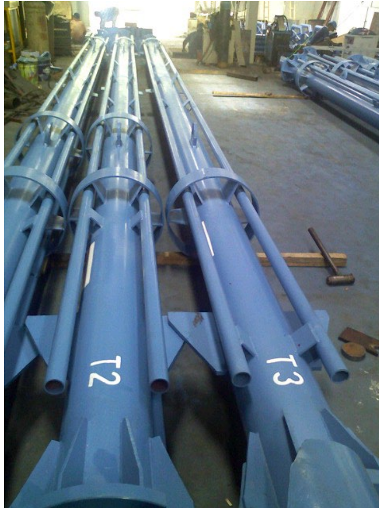
40FT x 10" Jetting Intermediate Section (Type 2 & 3)
