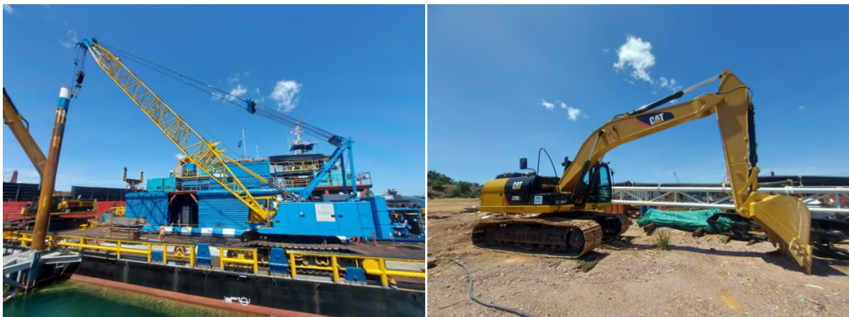
Figure 3-7 SCX900 (90T) Deck Crane and CAT320 Excavator (Convertible to Amphibious)
