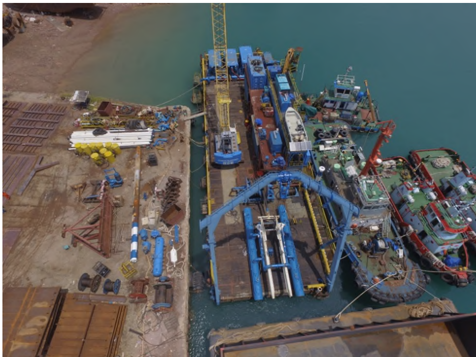
Figure 6-3 UB01 Miss Pennie rigged for Post Trench using Stern A-Frame
