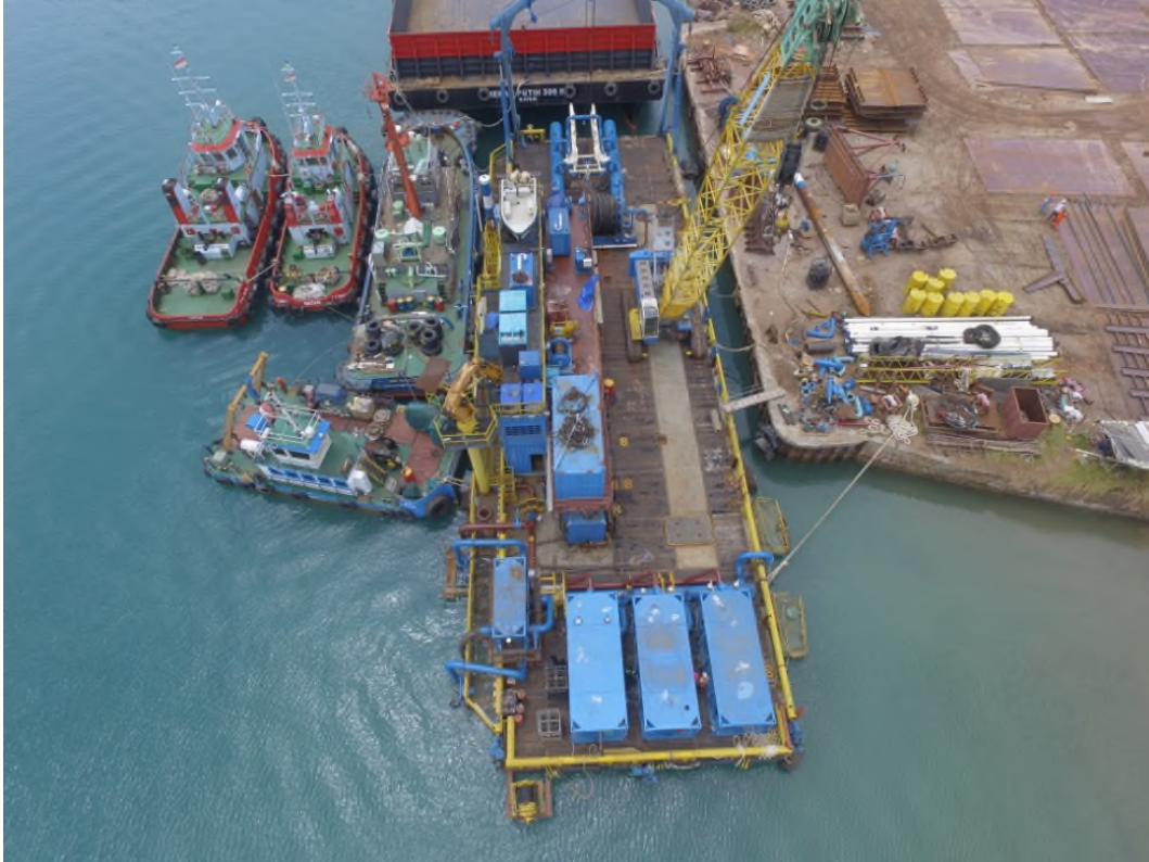
Figure 6-4 UB01 Miss Pennie rigged for Post Trench using Stern A-Frame
