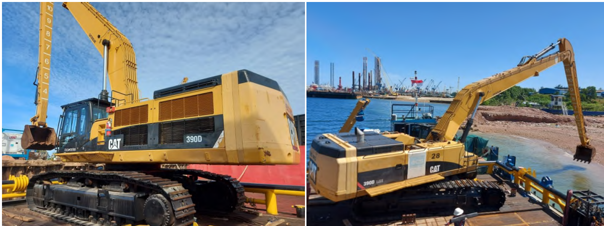
Figure 3-6 CAT390 Long Boom Excavators with 2m 3 Buckets
