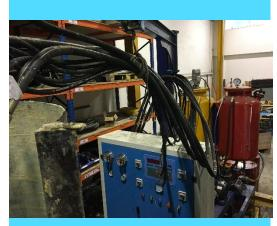
OCS owns 2 unit of PU Foam pump, a high pressure foaming machine used for the manufacture of polyurethane rigid, semi-rigid, soft foam such as insulation pipes, cold storage, thermal insulation, sound insulation, etc. The equipment has the advantage of high pressure mixing, precision proportion etc.
