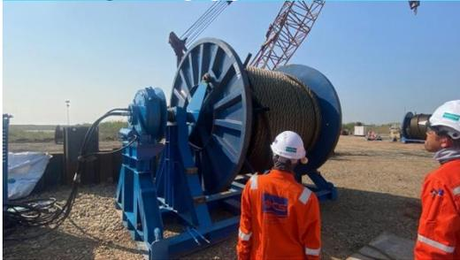
OCS owns different types of spoolers specified for various kinds of job scope. This particular wire Spooler is utilised for our pipe pull scope. The reels are interchangeable and can be replaced on site.
