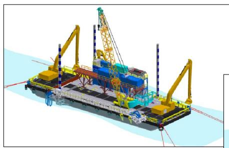
Trailing Arm can be used for trench maintenance and for water depths between 12 and 31m. The arm is equipped with high pressure jets and submersible dredge pumps and air lifts to remove trenched material.
